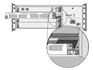
Figure 3-4. Installing the 7F06-02 Module in the 7C04 Workgroup SmartSwitch
